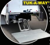
Designed so that the platform folds and stows under the truck body in dock ready position, the Tuk-A-Way is offered with a wide range of steel and aluminum platform configurations and various bed height options.
