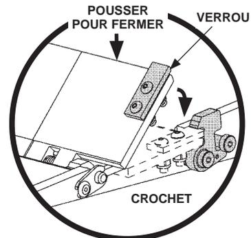
**FERMER LES BUTÉES D'ARRÊT DE CHARIOT (CÔTÉ DROIT DE L'ÉLÉMENT RABATTABLE)**
