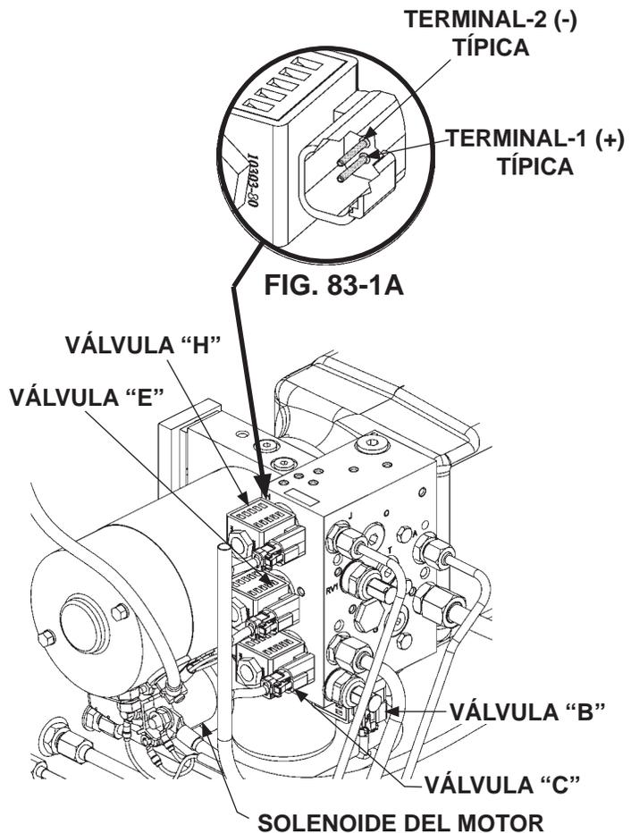
**VÁLVULAS DE BOMBA/MOTOR Y CONEXIONES ELÉCTRICAS PARA DESCENSO ASISTIDO (SE MUESTRA BOMBA DE DESCENSO ASISTIDO) FIG. 83-1**
