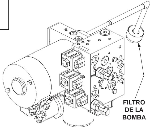
**ENSAMBLE DE LA BOMBA CON EL DEPÓSITO ELIMINADO**
