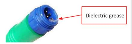
5. Align the keyed connectors and push together. Tighten blue ring until it is fully seated with no gap between the connectors. Grip both ends of connector firmly by hand and tighten.
