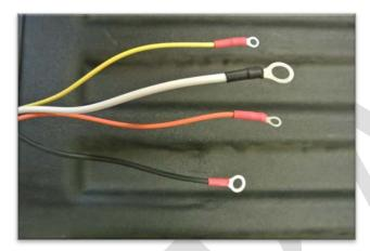
**STEP 19** Position the heat shrink over the crimps and apply heat to the 4 terminals.
