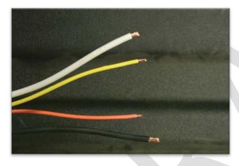
STEP 16 Strip 3/8 of an inch of insulation off all 4 wires.
