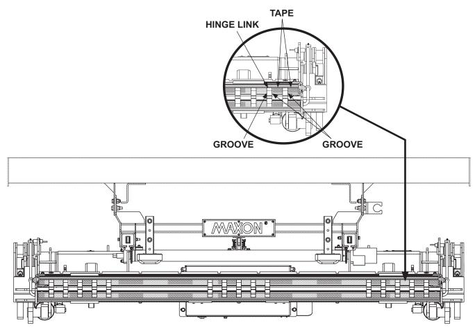
**CUTTING TAPE ON FLIPOVER HINGES** FIG. 5-1
