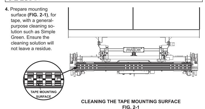
**NOTE:** Avoid touching the adhesive side of the tape to prevent contamination.
