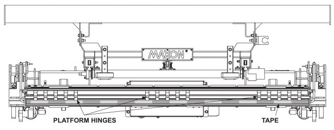
APPLYING THE TAPE TO PLATFORM HINGE FIG. 2-2
