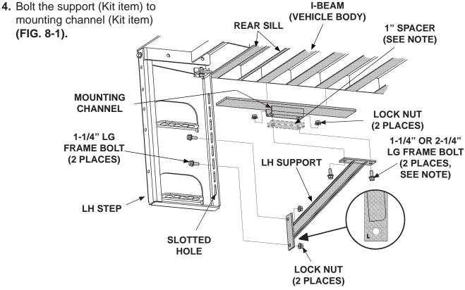
**BOLTING SUPPORT TO MOUNTING CHANNEL &** STEP (LH STEP & SUPPORT SHOWN) FIG. 8-1
