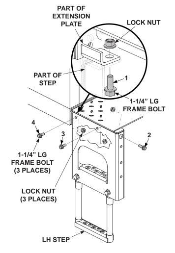
**BOLTING STEP TO EXTENSION PLATE** (LH STEP SHOWN) FIG. 12-1
