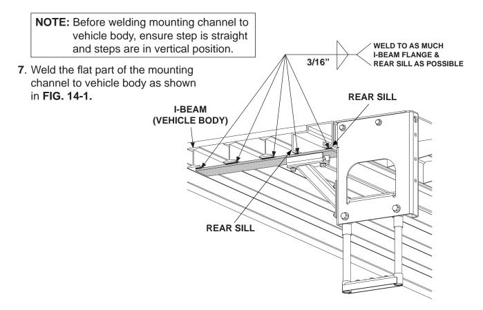
WELDING FLAT OF MOUNTING CHANNEL TO VEHICLE BODY (LH STEP SHOWN) FIG. 14-1
