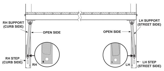
**CORRECT INSTALLATION OF** STEPS & SUPPORTS (REAR VIEW SHOWN) FIG. 5-1
