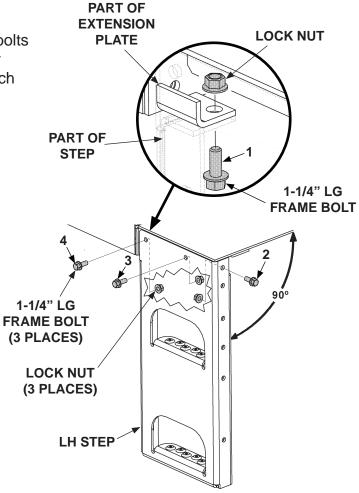
**BOLTING STEP TO EXTENSION PLATE** (LH STEP SHOWN) FIG. 7-1
