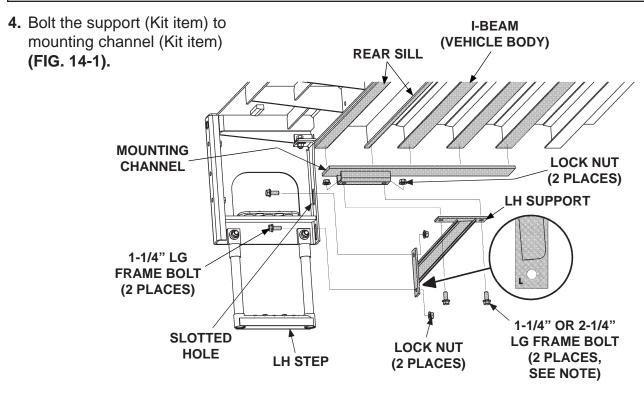
BOLTING SUPPORT TO MOUNTING CHANNEL & STEP (LH STEP & SUPPORT SHOWN)
