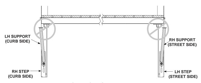
INCORRECT INSTALLATION OF STEPS & SUPPORTS (REAR VIEW SHOWN) FIG. 5-2
