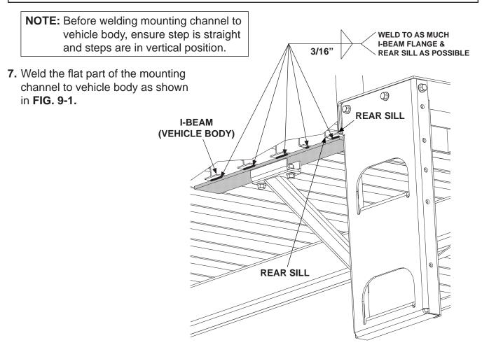
WELDING FLAT OF MOUNTING CHANNEL TO VEHICLE BODY (LH STEP SHOWN) FIG. 9-1
