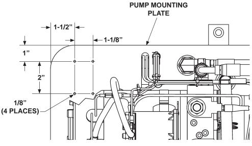
MARKING & DRILLING HOLES FIG. 3-1
