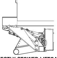
CORRECTLY STOWED LIFTGATE FIG. 2-1
