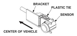
POSITIONING SENSOR IN BRACKET (RH SIDE SHOWN) FIG. 6-1
