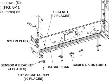
INSTALLING BRACKETS FIG. 8-1
