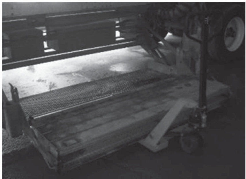
PLATFORM RUN ALL THE WAY PUT OUT & SUPPORTED BY PALLET JACK FIG. 2-3
