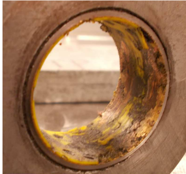
Example of wear/damage to liner
