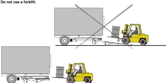
Only when the Slidelift is retractet under the vehicle.
