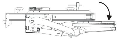
No contact between slideframe and platform
