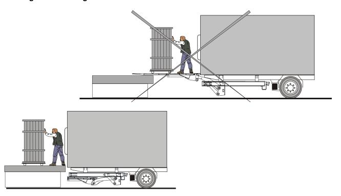
Only when the Slidelift is retractet under the vehicle.
