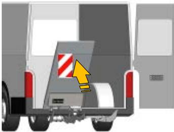
19. Close the platform with the operating panel (tilt-up) or the option 3-button handheld remote (tilt) + (lifting).
