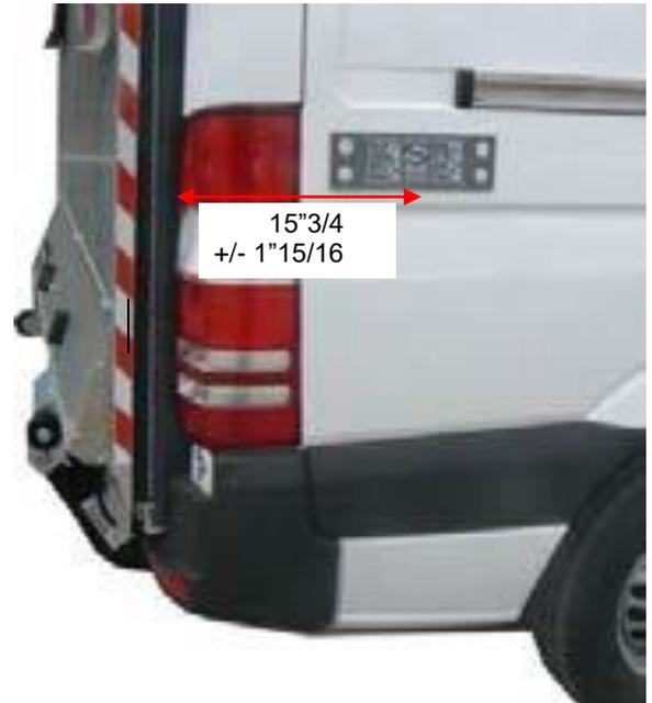
The control panel is mounted with 4 screws in the prescribed Distance (see drawing).
