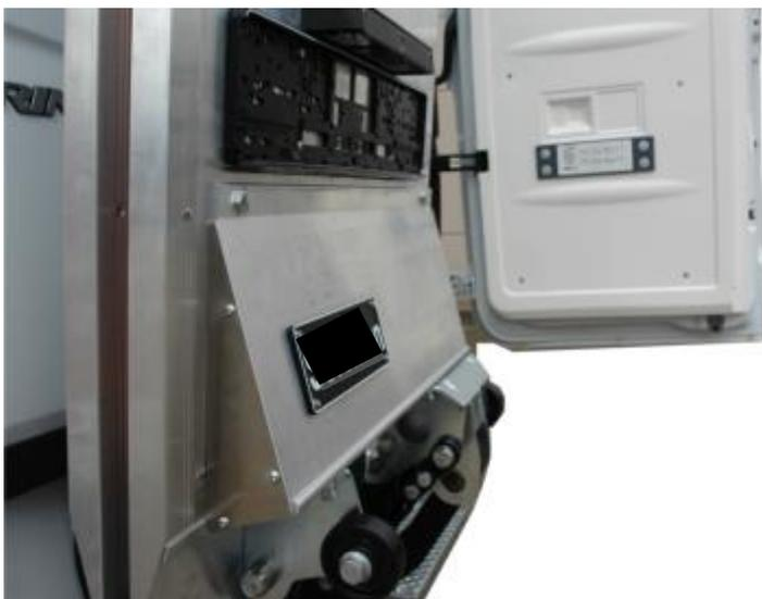
The control panel can be mounted on the inside of the right door.
