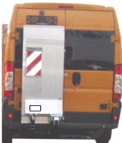
The number plate and the number plate lights on the vehicle is in some vehicles placed over the platform of the tailgate.
