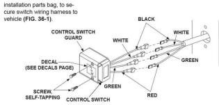
CONTROL SWITCH WIRING CONNECTIONS FIG. 36-2
