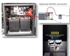
The complete system consists of a pre-installed DC/DC converter in the battery box (see picture) and either a Direct™ (connects to a single power source) or Select™ (can switch between multiple power sources) module that controls the system (please see chart below).
