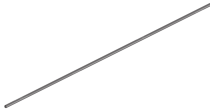
TORSION BAR, 93-1/16" LG. (KIT P/N 295486-01 ONLY) P/N 263041-21 QTY. 1
