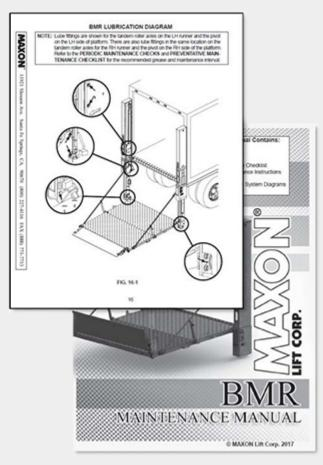
Many MAXON® liftgates manufactured today are equipped with grease fittings located at critical rotational points and bearing surfaces. It's of critical importance that these grease points are lubricated at the prescribed intervals as outlined in our maintenance manuals.
